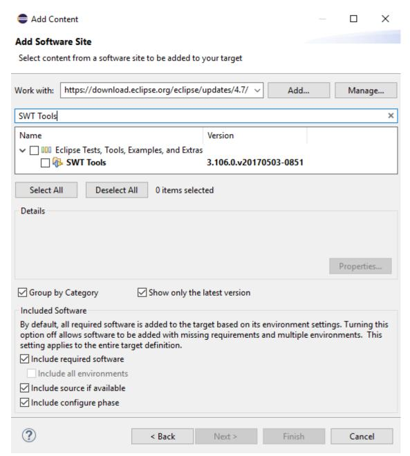
The wizard for adding new plug-ins to the target platform. Select the plug-in "SWT Tools" in order to add SWT spy to RCE.
